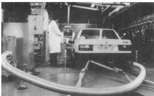
Figure 5. Vehicle dynamometer for the measurement of exhaust emissions.
