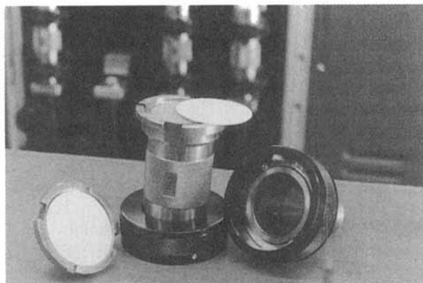
Figure 7. Detail of a filter to collect particulates during a vehicle test with a diesel powered passenger car.
