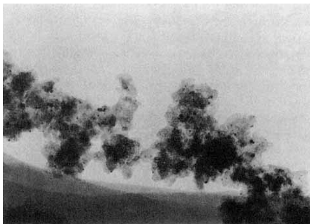
Figure 39. Transition electron microscope picture of precious metals on a washcoat particle.
